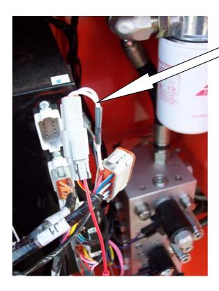
Plug the white jumper wire on the two pin supplied into pin hole #6 on J1 and plug the halves of the jumper plug together
