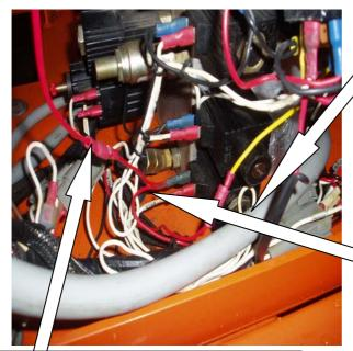
Crimp a male bullet terminal onto the red wire that goes back into the stabiliser loom and plug the red wire from the jumper plug into it.
