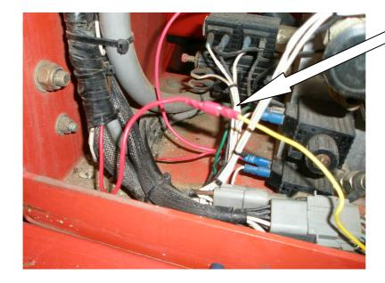
At the stabilizer manifold, locate where wire #9 is crimped together with the RED wire and cut wire # 9 off flush with the terminal.
