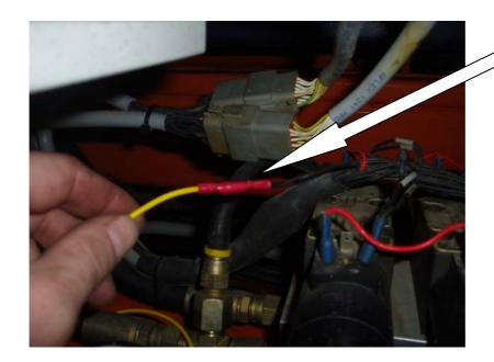
Crimp the male bullet terminal supplied onto wire 9 and plug it in the other end of the yellow wire supplied.
